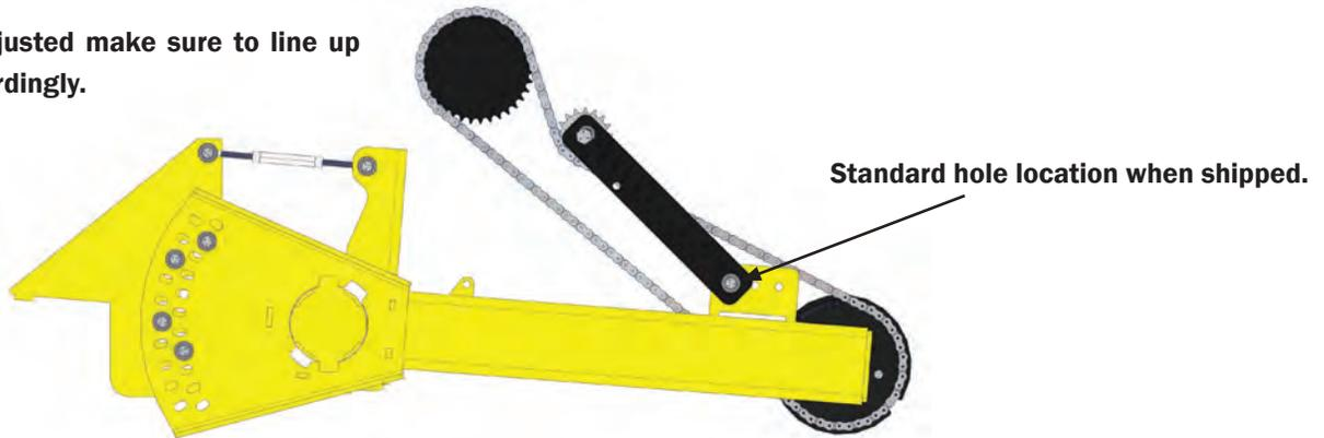
When desired location for arm is obtained, adjust turnbuckle until it is tight.
