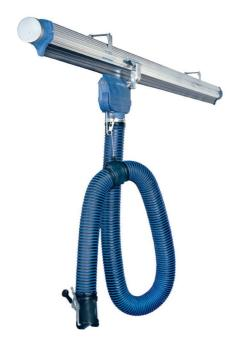
Efficient system for trucks, cars and vans in motion. With damper and shock absorber on trolley and safety coupling on exhaust hose for maximum operational safety. Available with automatic disconnection of the nozzle. The 920/1500 trolley is specially designed for moving vehicles. The maximum design airflow is 1500 m³/h (880 cfm) per trolley.
