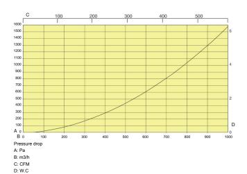
Pressure drop valid for 6 and 7 m track with 5 m hose, Ø 125 mm, and HB 600LL nozzle.
