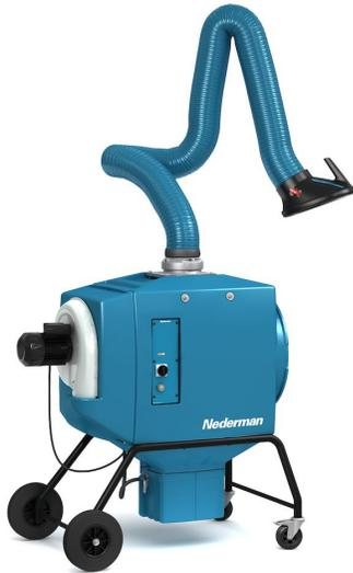
The FilterBox 10M is equipped with a N24 fan for a maximum air flow capacity of 1 000 m<sup>3</sup>/h (600 CFM). An integrated silencer reduces noise from the fan and outlet air.
