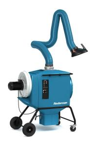
The FilterBox 12A is has a maximum air flow capacity of 1000 CFM (with NEX-HD arm) to maximize weld fume extraction. An integrated silencer ensures quiet operation. Advanced system controls allow for automatic cleaning when air flow is too low. Available either as a mobile unit on wheels or attached to a floor stand. Additional protection from harmful particles, for example, from stainless steel welding fumes, is provided if a HEPA filter is installed.
