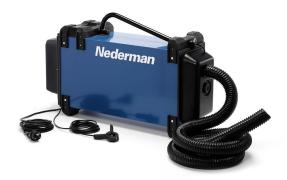
The Fume Eliminator is a portable welding smoke filter unit designed to be carried to the working area. Connected to a welding torch or to an extraction nozzle, the FE unit extracts the welding fume directly at source. FE 840 has a manual start/stop function while the FE 841 has an automatic start/stop function, which starts the unit as soon as the welding begins.
