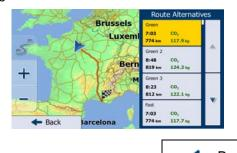
7. Select one of the route alternatives then tap and hold \_\_\_\_\_\_ for a few seconds to return to the Map screen. The software recalculates the route. The orange line now shows the new recommended route.
