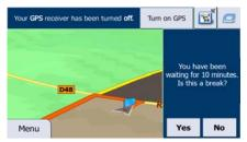
When a break is initiated, the continuous driving timer stops and it is reset to its default value, the daily driving timer also stops, and the break timer starts counting down (the break starts from the moment when the vehicle stopped). When the vehicle is in motion again, the break timer is reset, and both driving timers start counting down again.
