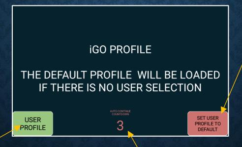
Default profile with configurations set by *GPSIS*. Note: the over speed warning is set to 105% of the current location speed limit.
