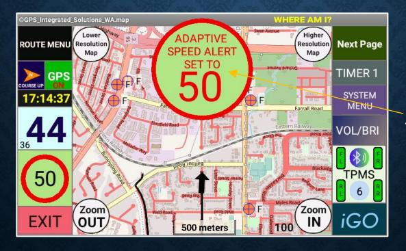
Adaptive message will be displayed when a new **Speed Alert** setting is calculated based on the vehicle speed and acceleration.
