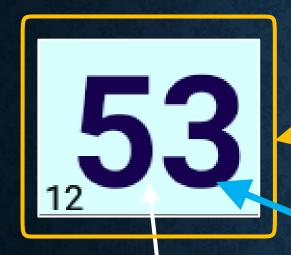
Vehicle Speed & Rolling 90s Ave. Short press to will disable the Adaptive Mode and set the User Mode to the current vehicle speed.
