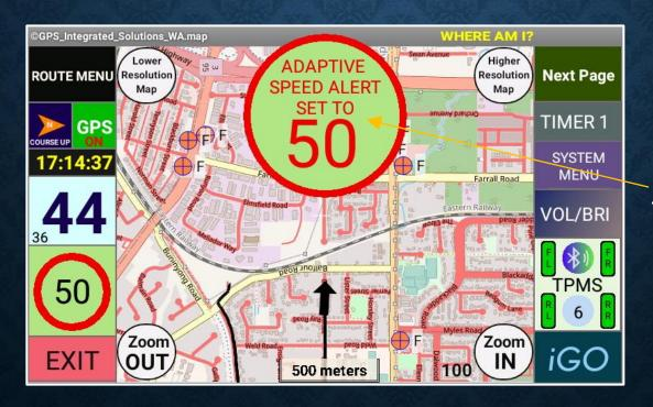
Adaptive message will be displayed when a new **Speed Alert** setting is calculated based on the vehicle speed and acceleration.
