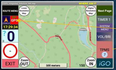
1. Turn the GPS receiver OFF & Drag the map to the desired location.
