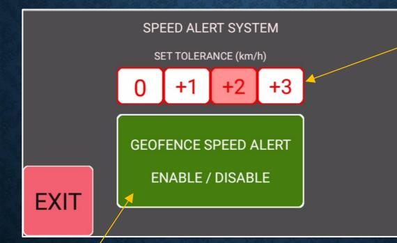
Set the tolerance value that will be added to the Speed Alert value.
