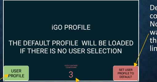
Default profile with configurations set by **GPSIS**. Note: the over speed warning is set to 105% of the current location speed limit.
