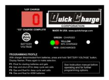
When AC power is applied, but the charge leads are not connected to the battery, or if connected reverse, A red/green alternating LED.
