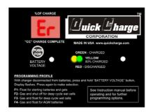
Error is displayed at the end of a cycle and a green/yellow alternating LED if a minimum voltage is not reached in the time given. See trouble shooting for more info.
