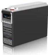
The leading advantages are a charge that is up to five times faster than the flooded version, and the ability to deep cycle. AGM offers a depth-of-discharge of 80 percent; the flooded, on the other hand, is specified at 50 percent DoD to attain the same cycle life. The negatives are slightly lower specific energy and higher manufacturing costs than the flooded.
