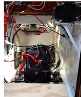
Now knowing my battery dimensions, I discovered that it was possible to design a battery box under the cockpit floor that would not require removal of the original braces for the cylindrical gas tank or the raw water thru-hull. The box has a 3/4 inch ply wood floor, with sides of 1/2 plywood, lined with EPDM pond
