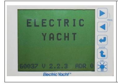
When power is turned on, the display will power up. It will say ELECTRIC YACHT across the upper part of the screen. The bottom line of the screen will show the firmware p/n and version number that is programmed into its microprocessor. It will also show its node address on the Electric Yacht RS-485 communication bus. Normally, this will show as **ADR 0.** If a second display is connected to the same bus, it needs to be set to **ADR 1**.
