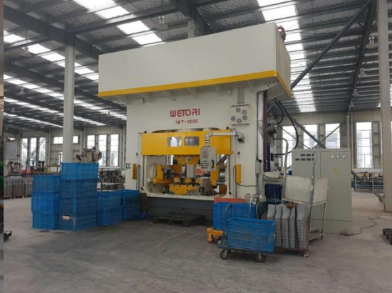
▲1000T Hydroforming Machine
