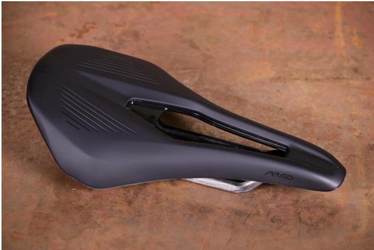
Saddles have different stack heights (distance from the rails to the top of the padding), for example, meaning that a new perch could leave you sitting higher than before. We're not talking about a couple of millimeters here; some saddles are well over a centimeter taller than others, and not many brands give you this measurement on their product information.
