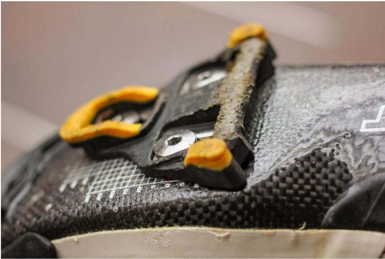
As a cleat wears, the position of your shoe on the pedal can alter. This can affect the alignment of your ankle, knee or hip and lead to problems.
