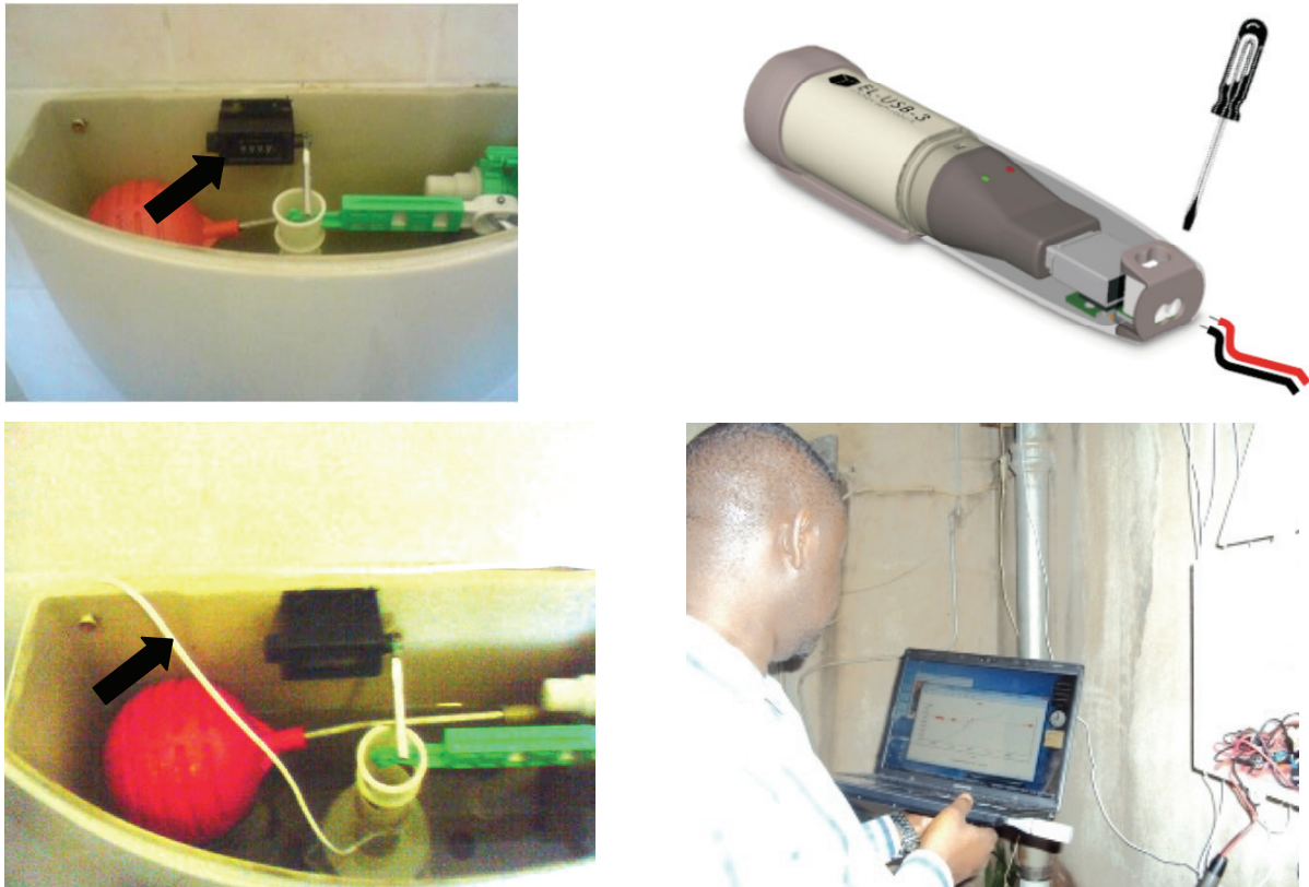
Figure 27. (Top left) A toilet cistern housing a manual counter with a lever; (Top right) An electronic data logger; (Bottom left) A probe from an electronic logger which measures voltage difference within water in the toilet cistern; (Bottom right) Downloading data from an electronic logger unto a computer.
