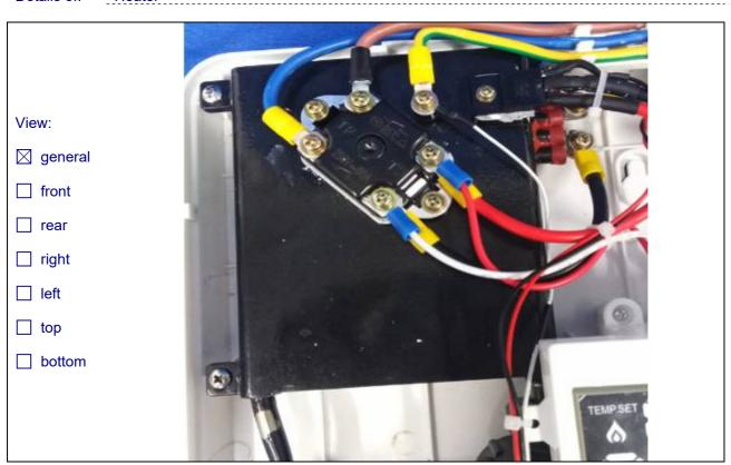
Details of: Thermal cut-out
