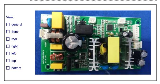
Details of: Main Control PCB backboard
