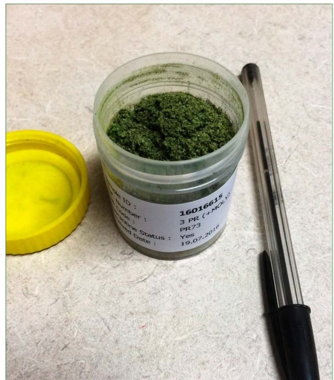
Figure 8 Screened and dried dry matter sample ready for dry matter analysis (image courtesy of AgVita Analytical)
