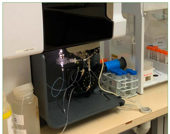
Figure 10 Inductively Coupled Plasma Spectrometry (ICP) instrument used for both dry matter and sap analysis - top full ICP set up, middle automated sampling, bottom ICP analysis (images courtesy of AgVita Analytical)
