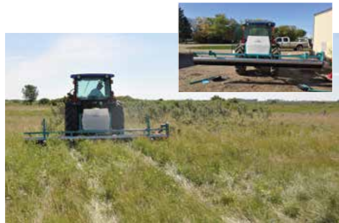
Weed wiper used to apply the chemical to the western snowberry. The weed wiper allows us to target the snowberry only.
