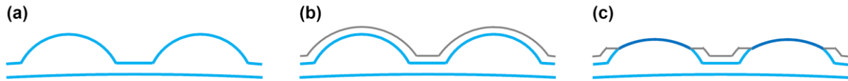
Fig. 1 Generation of gap-masked lens array on curved substrate. (a) SFLA; (b) spray coating on the SFLA; (c) finish cutting of lens array.
