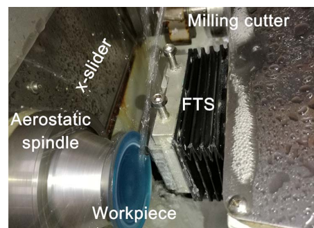
Fig. 9. Diamond machining of the PAL rear surface with the FTS.
