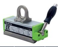
Ideal for thin sheets or parts, tanks/containers and thin-walled pipe that normally can't be lifted with a permanent, On/Off magnet. The magnetic field on the FXP is concentrated and shallow to drive the strength into thin material.
