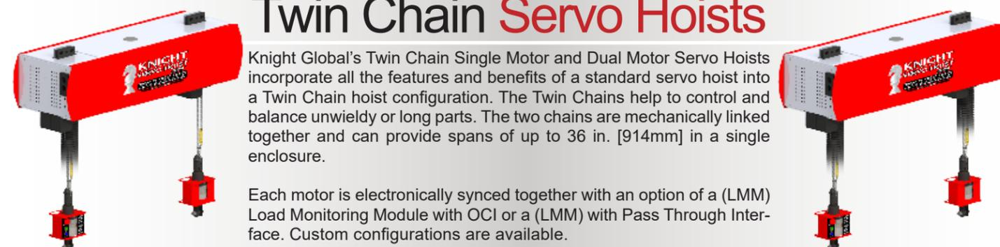
Knight Global's Twin Chain Single Motor and Dual Motor Servo Hoists incorporate all the features and benefits of a standard servo hoist into a Twin Chain hoist configuration. The Twin Chains help to control and balance unwieldy or long parts. The two chains are mechanically linked together and can provide spans of up to 36 in. [914mm] in a single enclosure.
