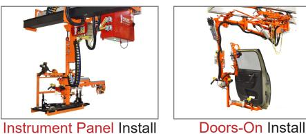
Servo Actuator, clamp style end effector operated by a programmable PLC system that controls the precise position and angle of the door for installation onto the vehicle.
