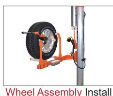
Nesting and manual clamp end effector mounted on an ATA4000 vertical mast arm. Fixture assists operator in picking up wheel assembly and rotates tire for install.
