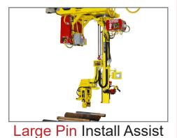
Vertical KSHVAR XYZ Roller Servo Hoist Arm using a hydraulic clamp style end effector that clamps, lifts 500 lbs. machinery pins and transfers into 300 degree hardening ovens.
