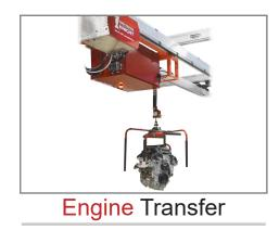
Hook style end effector operated by a XYZ Servo Hoist and Tractor system. System assists operator in moving the large engine from the line conveyor to the dunnage.
