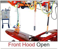
Vacuum style end effector operated by a programmable PLC system that controls the Air Balancer and Electric VFD Tractor that automatically attaches and raises the hood to operating level.
