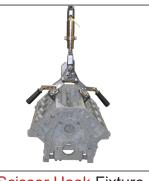
**Scissor Hook Fixture** Scissor hook style fixture that is suspended by a Knight Pneumatic Balancer. Transfers engine block from assembly line to the inspection workstation.
