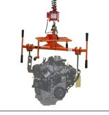
**Dual J-Hook Fixture** Dual J-hook style fixture operated by a Knight Servo System. Transfers engine from assembly line to the vehicle for installation.
