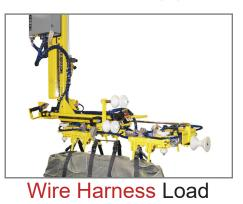
Clamp style fixture mounted on a vertical mast arm that loads, opens and spreads out the wire harness bag inside the vehicle cab.
