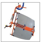
**Nesting Clamp Fixture** Nesting clamp style fixture suspended by a Knight Pneumatic Balancer. Transfers the hood from dunnage to the vehicle for installation.
