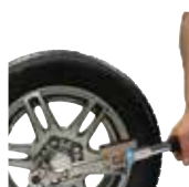
Completion of tightening process with Blue signal.
