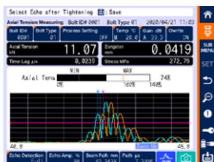
Waveform before &amp; after giving loading
