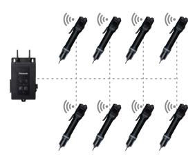
By using the optional Controller management software, data for up to 10 controllers (up to 80 tools) can be automatically collected and collectively managed.
