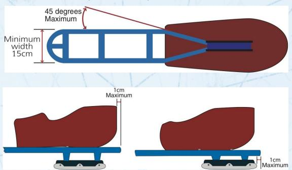
The front of the sled shall have a continuous curve with a maximum radius one half (1/2) of the inside width of the frame at its widest point forward of the seat. The following materials may be used in constructing this piece: Steel; Aluminum; Titanium; Magnesium, Polyurethane.
