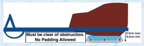
A plate or any kind of device covering the space between the sled frame side rails is not permitted.
