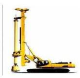
Two sets of Rotary Piling Rigs for doing larger piles like 1 meter & 1.2 meter dia
