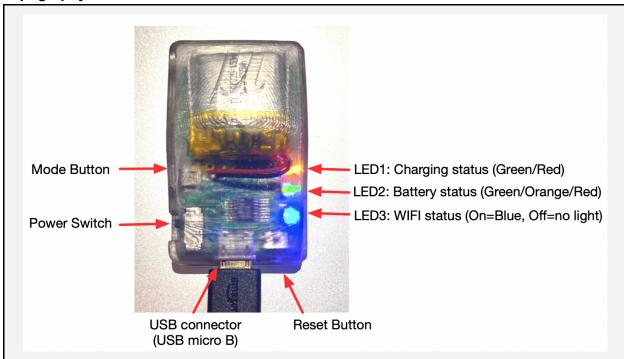
**USB connector:** We recommend to charge MUGIC<sup>™</sup> before use (this will take approximately 1 hour). MUGIC<sup>™</sup> will immediately begin charging when plugged into a USB power source supplying **5V with at least 500mA**. The device requires at least 5 minutes of charging before being able to be powered on, if the power is critically low.
