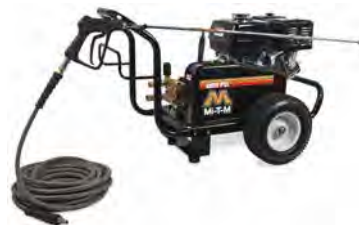
JCW Series Gasoline Belt Drive - 4000 psi, 3.5 GPM, 389cc
