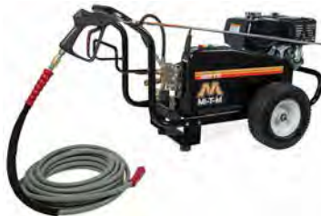
CW Premium Series Gasoline Belt Drive - 4000 psi, 3.5 GPM, 389cc
