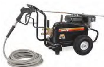
JCW Series Gasoline Belt Drive - 2400 psi, 2.8 GPM, 196cc
