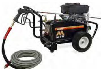
CW Premium Series Gasoline Belt Drive - 4000 psi, 4.0 GPM, 480cc
