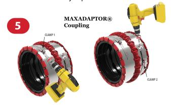
Tighten both sides of the MAXADAPTOR® Coupling, alternating back and forth.
