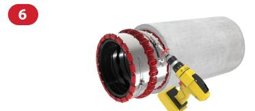
When the coupling ID's are closely matched to the pipe/adaptor OD's, install the MAXADAPTOR® Coupling onto the ShuvlNose® Adaptor. Take up all slack in coupling with a cordless drill or socket wrench.
