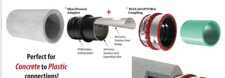
Transition is made by joining the **inside diameter of the concrete pipe** with the **outside diameter of the plastic pipe**.
