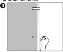
**STEP 3:** Attach the side locking strips around the frame leg. Repeat for remaining leg.
