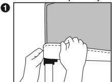
Single wall should be attached BEFORE Kanopy is staked down and Kanopy frame SET to the highest leg position. *Single wall can be attached to any side desired.*
