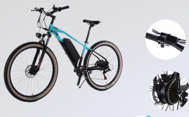
Frame Material: Aluminum Alloy Power Supply: Lithium Battery Battery Capacity: 7/10.4/13/17.5AH Battery Position: External battery Motor Position: :Mid-set motor/Rear Front fork: Spring/Oil fork/Gas fork
