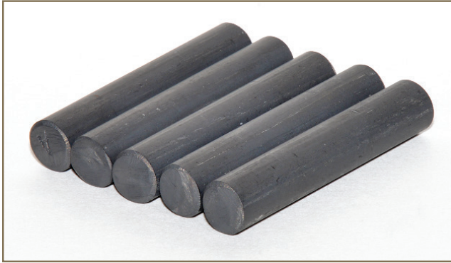
Fig. 2. FNC test part with post-oxidation in air
