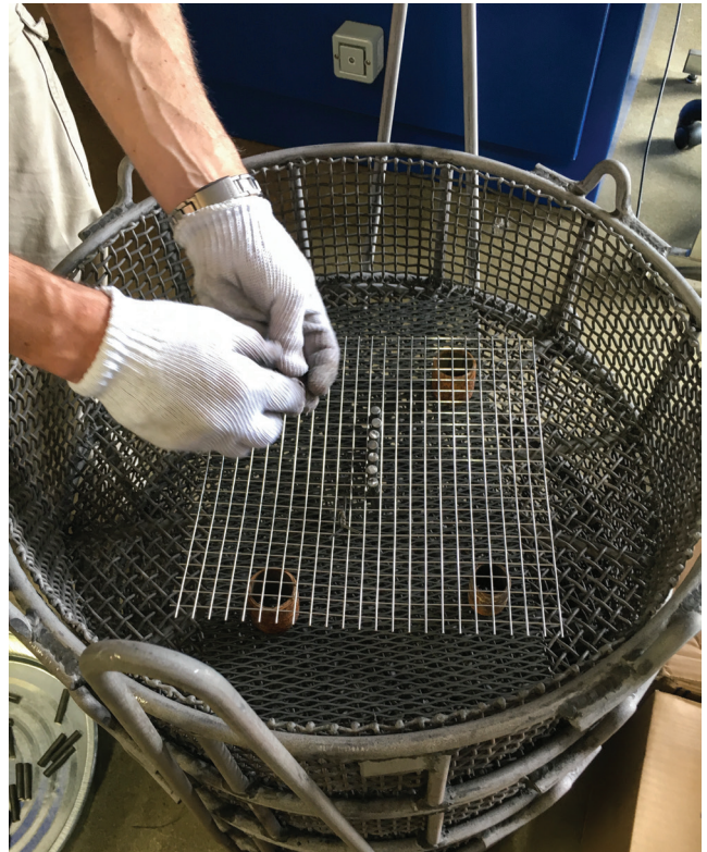
Fig. 4. Two sets of FNC test parts in a sealed pit furnace with an ammonia, nitrogen and \text{CO}_2 atmosphere.
