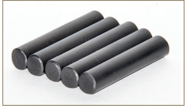
Fig. 3. FNC test part with post-oxidation in air with RPO
