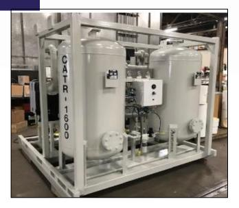
Designed for the rugged demands of the rental industry. Air Dryer Supplier, Inc. CATR Series, delivers clean, dry air, all in one complete, reliable package. Skid package includes an air cooled after cooler, bulk moisture separator, coarse pre filter, fine pre filter, heatless regenerative desiccant dryer and particulate after filter.
