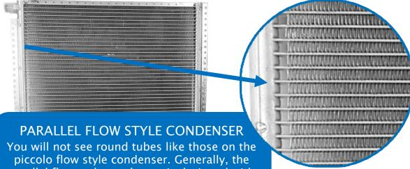
You will not see round tubes like those on the piccolo flow style condenser. Generally, the parallel flow style condenser is designed with more tubes with much smaller (less than 1mm in diameter) internal passages.
