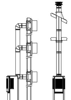
\* The H15 can be vented horizontally with the AstroCap™ system. For rear vent applications, H27 and H35 require a riser vent.
