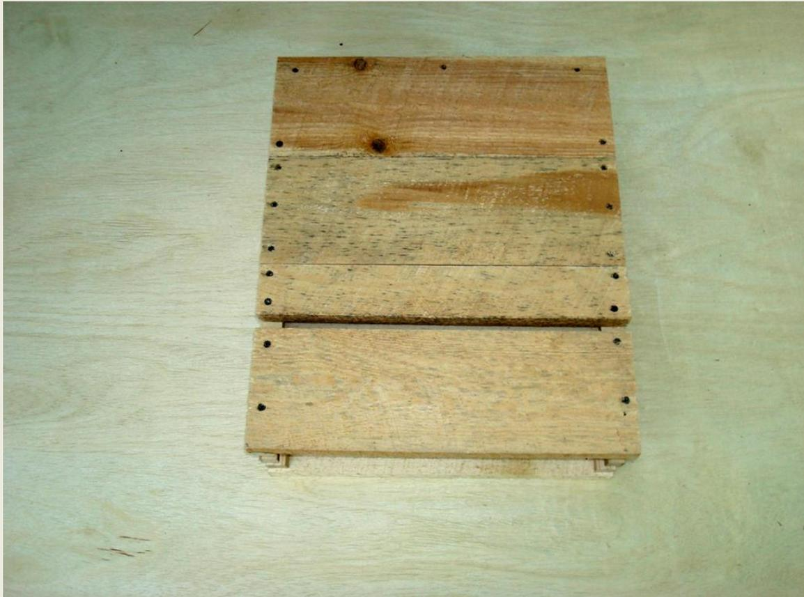
**The front is all pre-drilled and attached with 2" drywall screws.**
