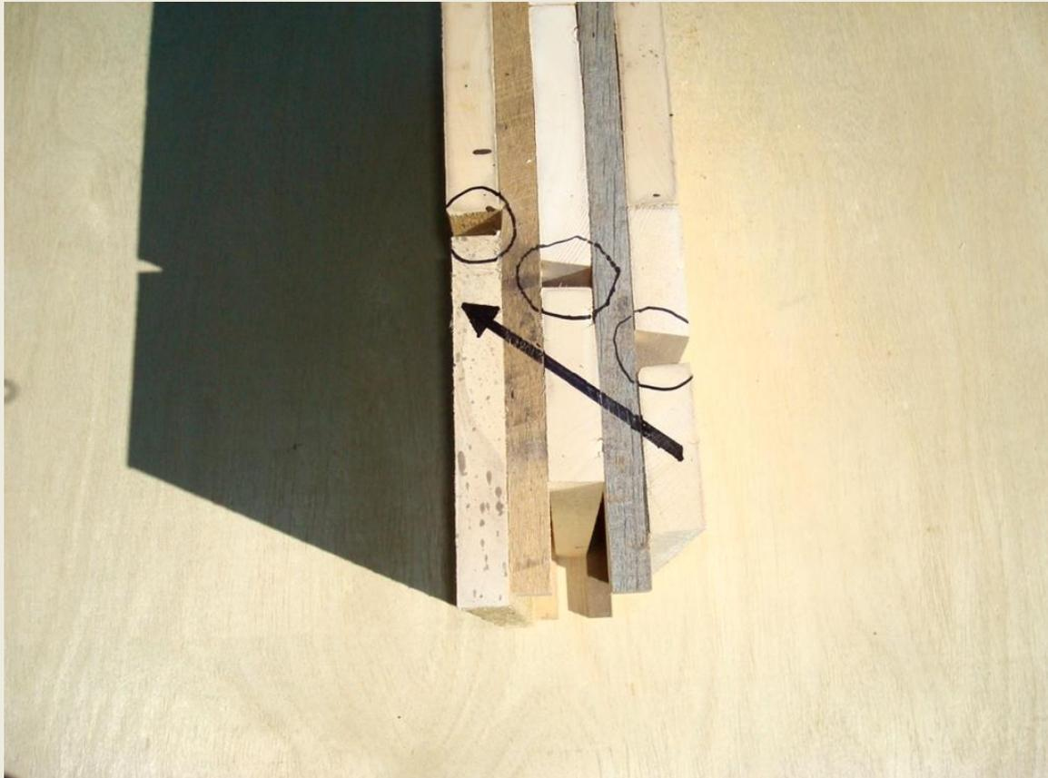
**Internal access gaps go upwards from the front to the back of the box.**
