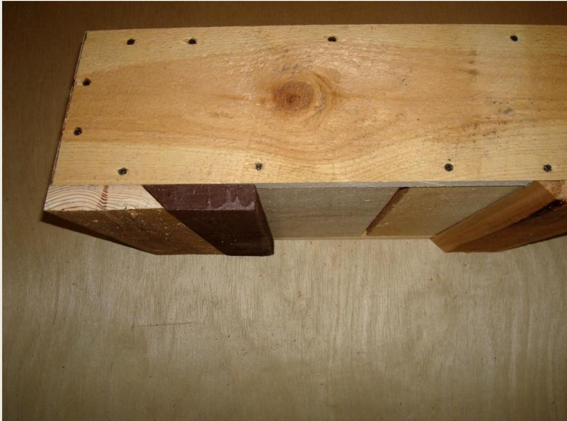
**The matching french cleat to be attached to the pole later.**
