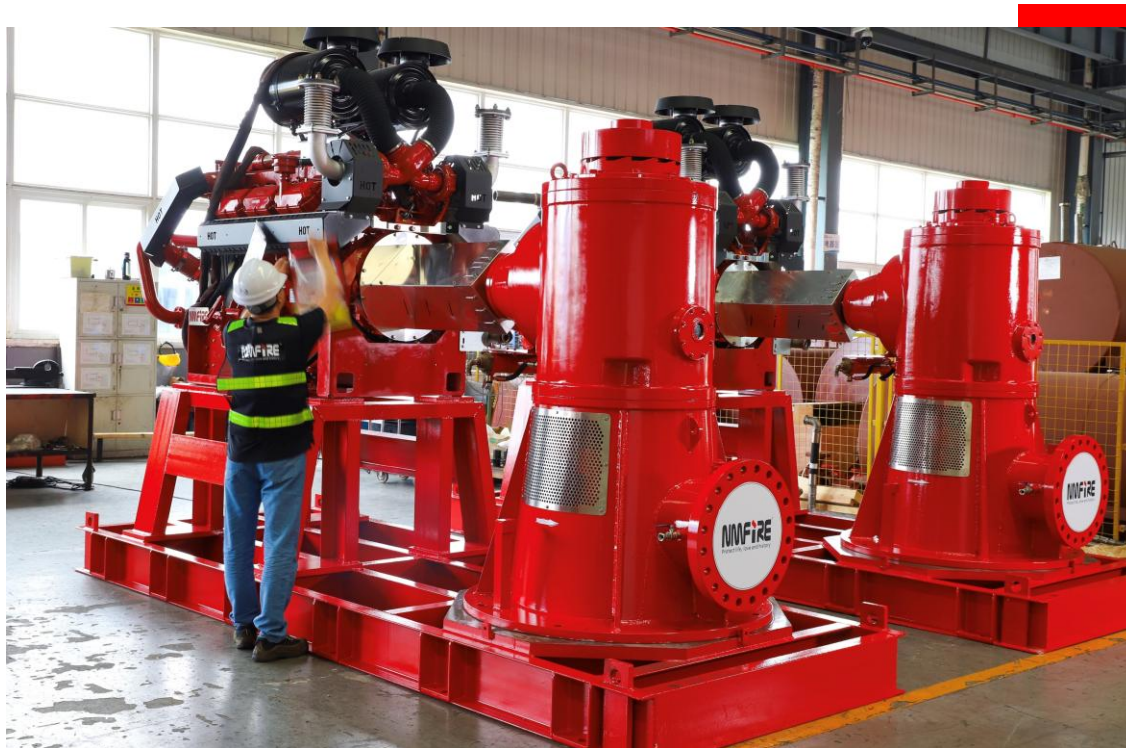
Vertical Turbine Pump, Engine : 1250 GPM, 130 PSI Jockey Pump : 12.5 GPM, 140 PSI
