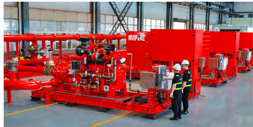
Diesel engine driven horizontal split-case fire pump package for Kuwait Oil Company (KOC) 发往科威特石油公司（KOC）的柴油机驱动中开泵撬装机组
