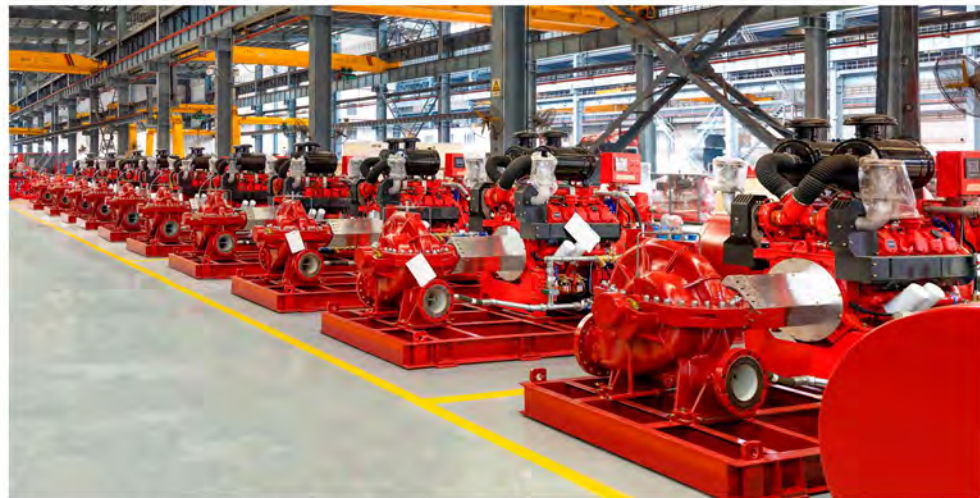
Diesel engine driven horizontal split-case fire pumps for oil and gas industry project in Nigeria 发往尼日利亚石油公司的柴油机驱动中开泵
