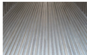
Refrigerated Container - Grilled Floor
