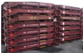
Flat Racks - Folding walls allow stacking
