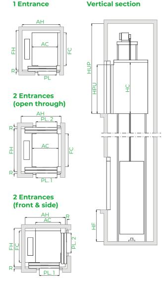
\*Note: The diagrams are for guidance only. Dimensions for 1 entrance. Car width and depth variable, in 5 mm increments. For simplification, table samples show increments of 100 mm.
