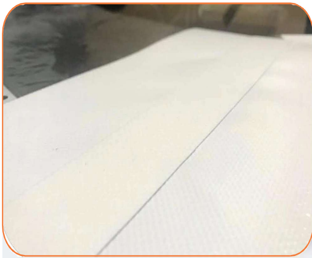
Normal Welding Bump Polyester Fabric Exposed
