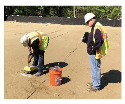
Scott Lukowski, a project engineer from DYMAR, does a compaction test, overseen by a worker from Connecticut Materials Testing Laboratory.
