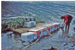
Above: Duncan McColl reads the anchors on the raft, after they have been loaded with a wheelbarrow.
