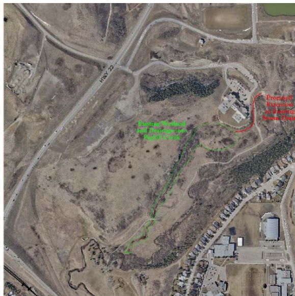
Above: This is a draft plan for a remediation project to divert flows from the storm water drainage. The plan would involve the extension of the existing outflow location.
