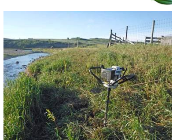
Above: This gas powered earth augur was the best choice of equipment for the task at hand. Although the ground was very dry and hard, a power augur worked best for creating a hole down to the proper depth. Hand tools would have made the job very difficult for this part of the planting.
